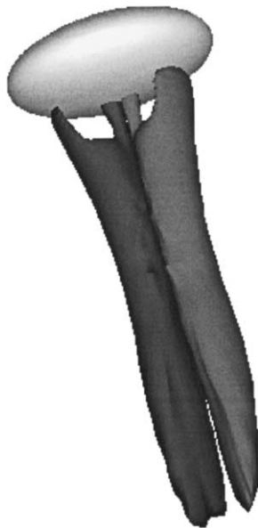
Fig. 3. Isosurface \omega_x R_{\text{eq}}/U_\infty = \pm 0.7 of the streamwise vorticity in the wake of an ellipsoidal bubble ( \chi = 2.5 , Re = 835 ).
